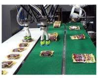
The Spider 300v is a two-robot case loading system with vision allowing processors and co-packers to pack both vertical and horizontal on the same line at the same time. This versatile packaging solution allows for random product arrival at high speeds; providing great flexibility in packaging formats. Bulk, variety, display and single flavor packing are all achievable! Built for high speed packing and quick changeover between recipes, the Spider 300v is capable of handling standard RSC
